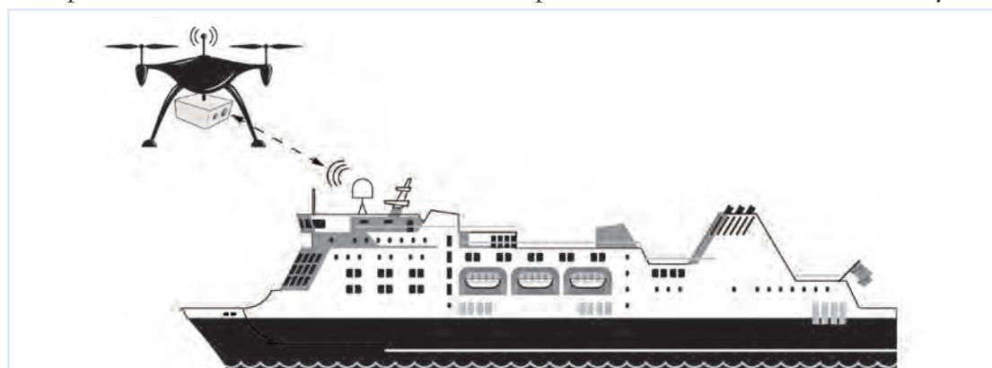
Figure 10: the Drone Satellite Simulator is maneuvered so it aligns with the ship’s antenna prior to testing. By then maneuvering the drone the operator can easily test the terminal’s satellite tracking.
